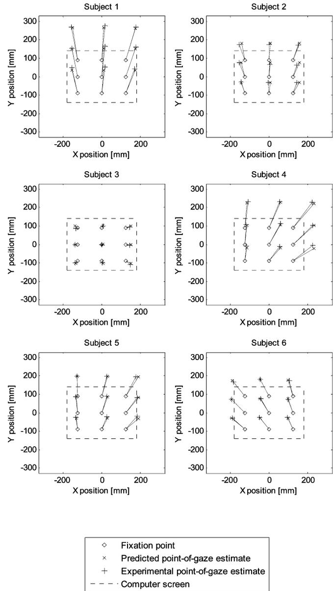
Fig. 3. PoG estimates predicted analytically as compared to the experimental estimates.
