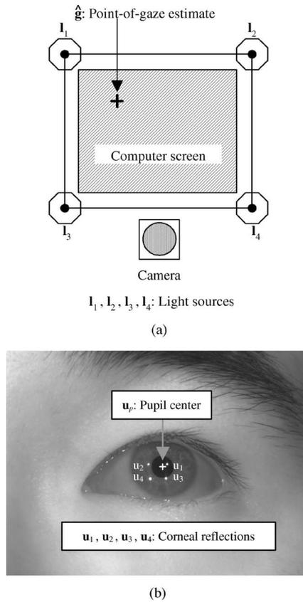
Fig. 1. (a) System setup with four light sources positioned around a computer screen, and a camera under the screen. (b) Image of the eye as captured by the camera, showing the four corneal reflections and the pupil center.
