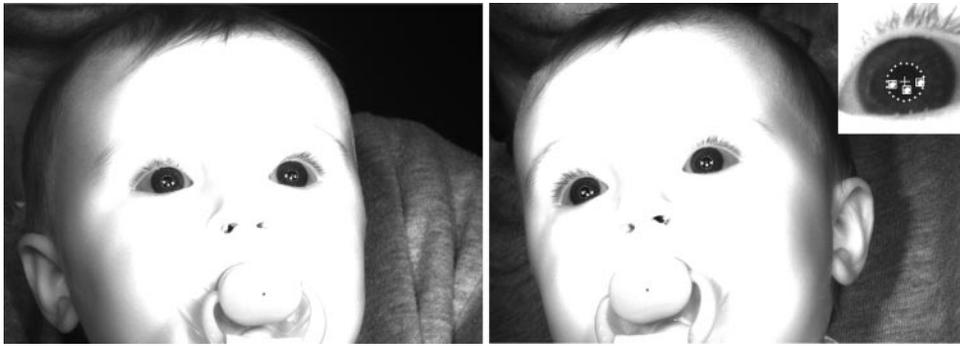
**FIGURE 1.** A pair of images of an 8-month-old infant from the remote binocular gaze-tracking system. Pupil center and three corneal reflexes (virtual images of the system's three infrared light sources) are identified and tracked automatically by the system (*inset*).
